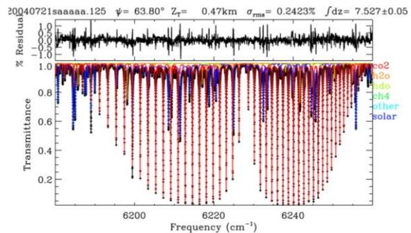
Figure 4 Spectral fit to the  $6220\text{ cm}^{-1}$   $\text{CO}_2$  band
