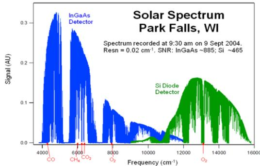
Figure 3 Typical TCCON FTS spectral domain
